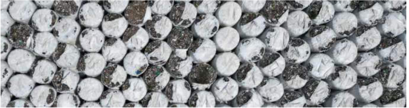
Photo 15 13/12/23 13:19hrs. Breaking of the bale covers and vegetation growth seen on the bales.
