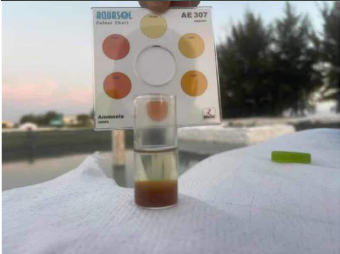
STARTED DISCHARGE. WATER QUALITY MEET DEWATERING PARAMETER.
