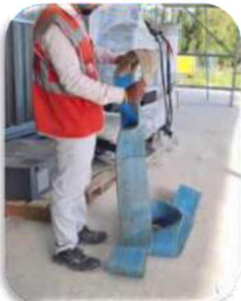
Lifting slings Inspection
