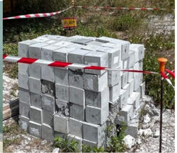
Photo 41 15/01/24 – Concrete test cubes kept in curing tank, tested cubes collected and kept for disposal.
