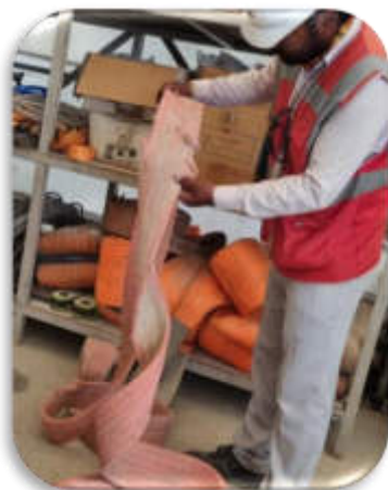
Lifting slings Inspection
