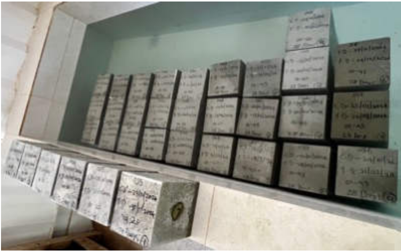
Photo 41 15/01/24 – Concrete test cubes kept in curing tank, tested cubes collected and kept for disposal.
