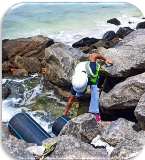
Dewatering Effluent Sampling
