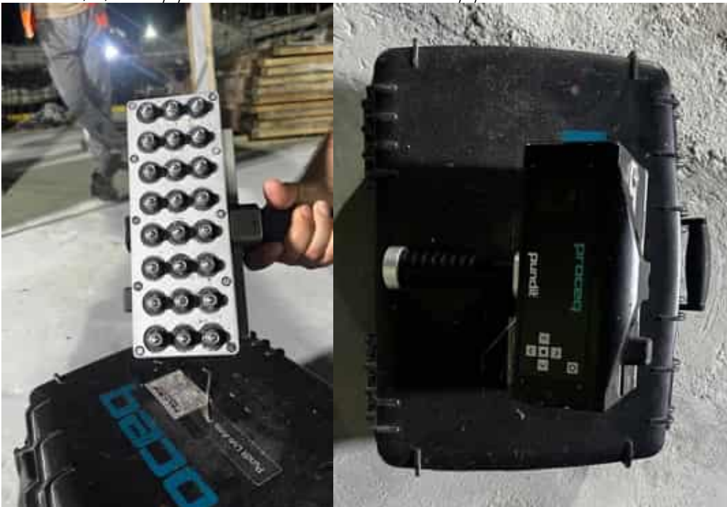
Photo 08 08/04/24 – Pulse Echo Ultrasonic test equipment used by the third party inspectors Falcon Laboratories.
