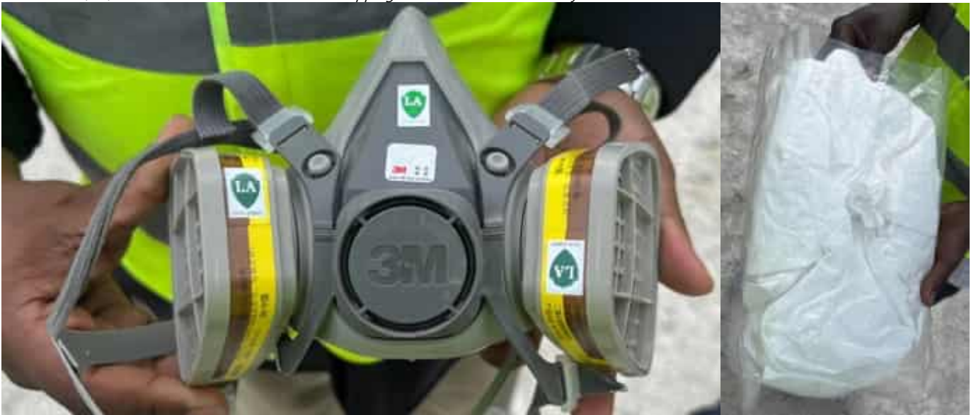
Photo 13 14/04/24 – Protective masks and disposable protective coats used by Villa staff for handling chemicals.
