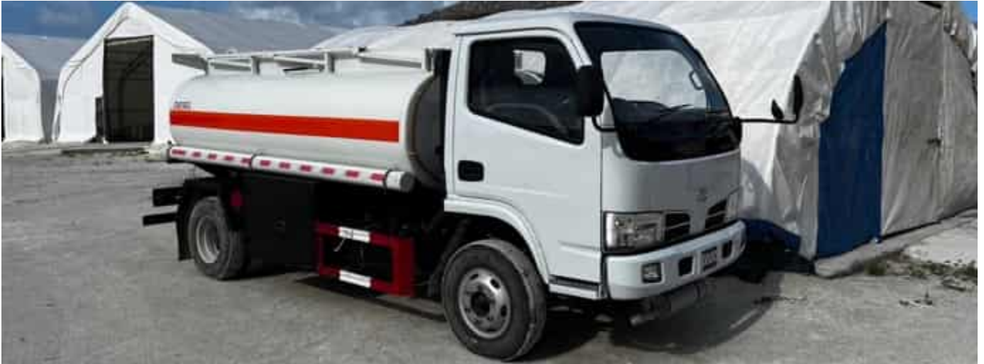
Photo 18 14/04/24 – Diesel tanker on site 5000litres capacity - Not registered and used outside site boundary to go to fill station, necessary steps should be taken for registration and safety signage should be in accordance to regulations.
