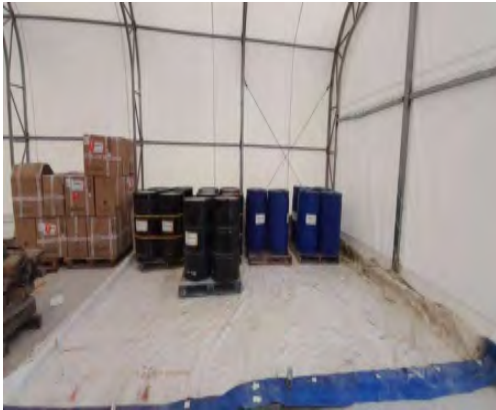
Figure 4: Inadequate Secondary containment provided and spillage observed in temporary storage tank of chemical in ware house area found during visit for inspection in mid of July.
