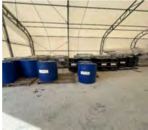
Figure 4: Inadequate Secondary containment provided and spillage observed in temporary storage tank of chemical in ware house area found during visit for inspection in mid of July.
